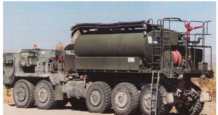
Military water distribution truck with 3,000-gallon tank.
